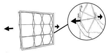
Once the frame has expanded fully push the two sides of an hook on each cross section so that you can hook the frame secured firmly in place.
